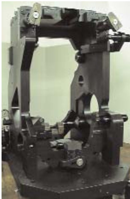
A single operation fixture for "Pump Housing". This fixture uses six locators, three clamps, two work supports, two pusher style clamps, two roller pushers and an equalizing mechanism, resulting in excellent Cpk readings.
