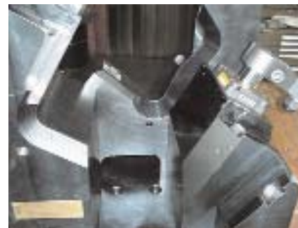
A close-up view of a fixture nest that holds an "Axle Housing."
